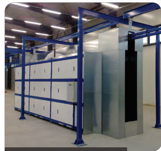
Most commonly, MDF powder coating systems use conveyor designs to move panels through pre-heat, powder application, curing and cooling stages. Photo courtesy: Heraeus-Vulcan.
