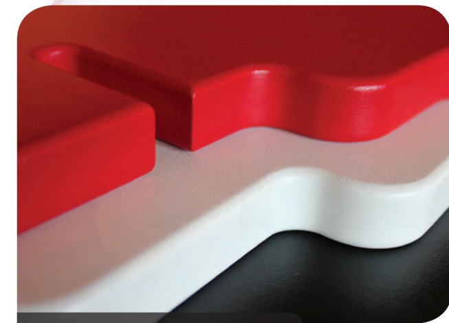
With powder coating, MDF panels achieve a hard, durable finish, even on edges and complex curves. It is important to use high-quality MDF board, to pretreat with heat, and to control cure times precisely. Photo courtesy: Heraeus-Vulcan.
