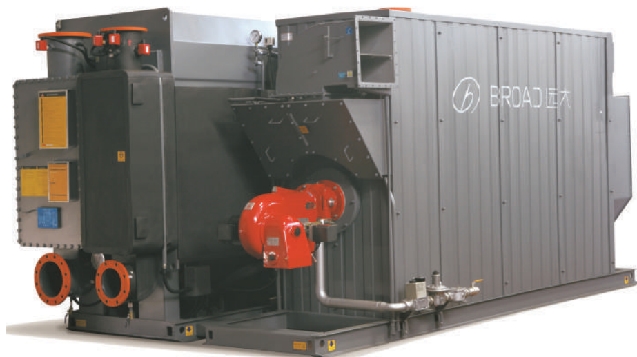
Direct-fired chiller from Broad U.S.A. in sizes from 40 to 3,300 tons provides building or process cooling as well as heating and hot water. This unit is available with a dual fuel (natural gas/oil) burner and features NOx emissions less than 10 ppm. Photo courtesy: Broad U.S.A.
