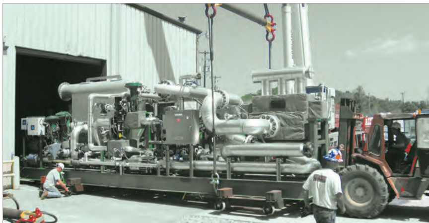
One intriguing option nearing commercialization is a heat recovery module by Echogen that uses CO 2 as a working fluid to extract a high proportion of heat from industrial and utility exhaust streams. The system is skid-mounted and operates in the range from 500° F to 1200° F. Courtesy: Echogen.
