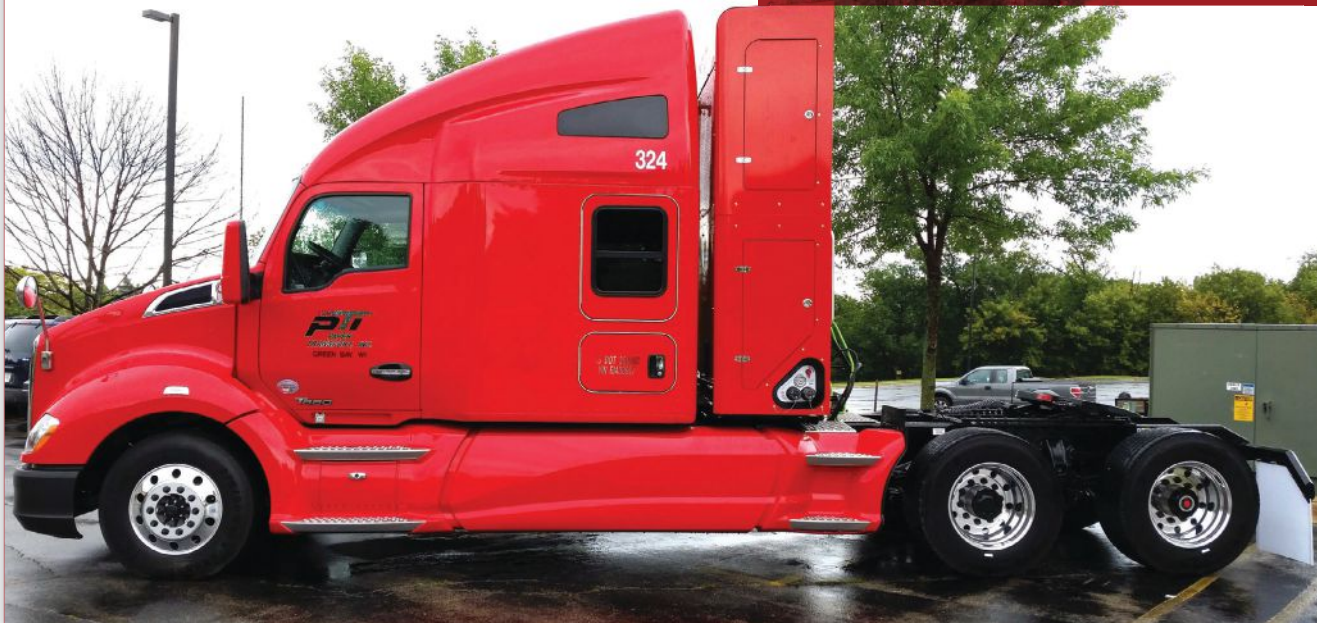
Kenworth road tractor with CNG storage tanks behind the cab. Photo courtesy: Agility Fuel Solutions
