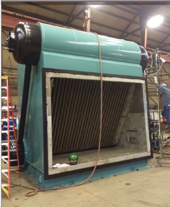
Photo illustrates the inlet side of the heat recovery gas generator at the University of Arkansas. Photo courtesy: Cleaver Brooks
