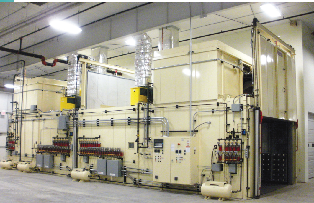
Batch-type ovens are used in a variety of applications, typically when required residence times are long. These units are often equipped with track systems for moving product in and out. Courtesy: Wisconsin Oven Corp.
