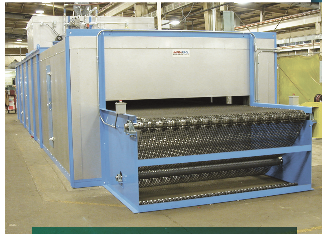
Conveyor ovens may use various methods for continuously moving product through various temperature heating and cooling zones. System include racks, trays, and suspension systems often used with powder paint. Courtesy: Infracor, Inc.
