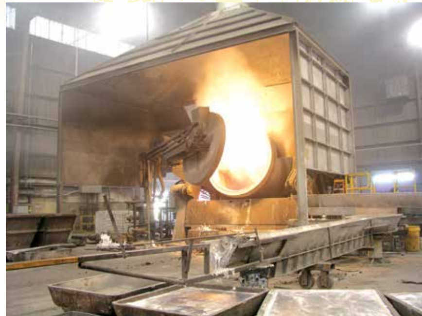
Oxy-fuel firing, as at this Kentucky aluminum recycler, reduces energy consumption. Photo courtesy Owls Head Alloys.
